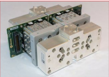
▲ Fig. 1 Taurus 16 (AA033) E-Band power amplifier.
