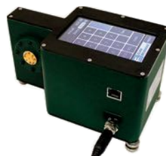
D band Programmable Attenuator 0-90dB functionality
